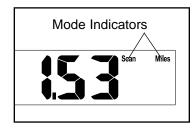
the scan mode is selected, and a second mode indicator will show which mode is currently displayed. Note: If a different mode is selected, you can select the scan mode again by repeatedly pressing the Display Mode button.
